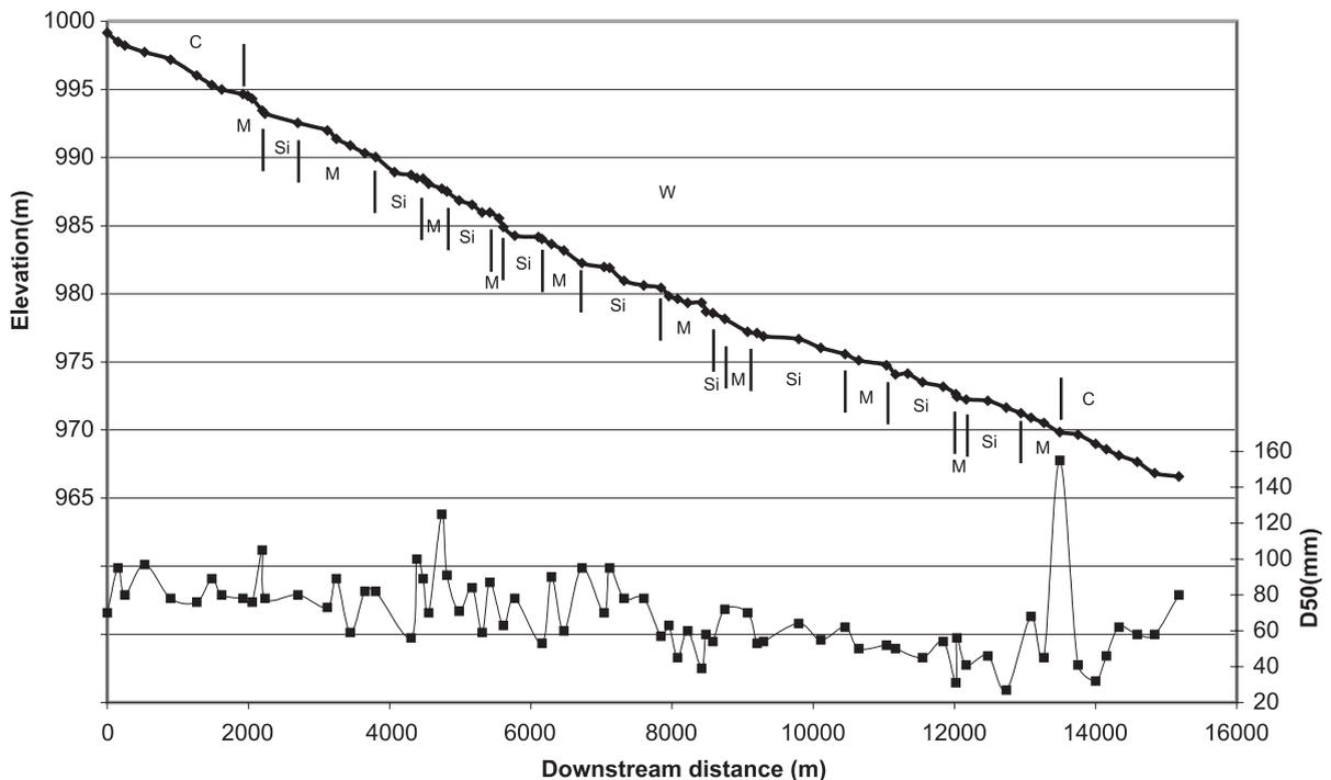
Fig. 2. Long profile and bed  $D_{50}$  for the confined and wandering patterns of the Renous River. Locations of confined (C), wandering (W) single (Si), and multiple (M) are denoted.
