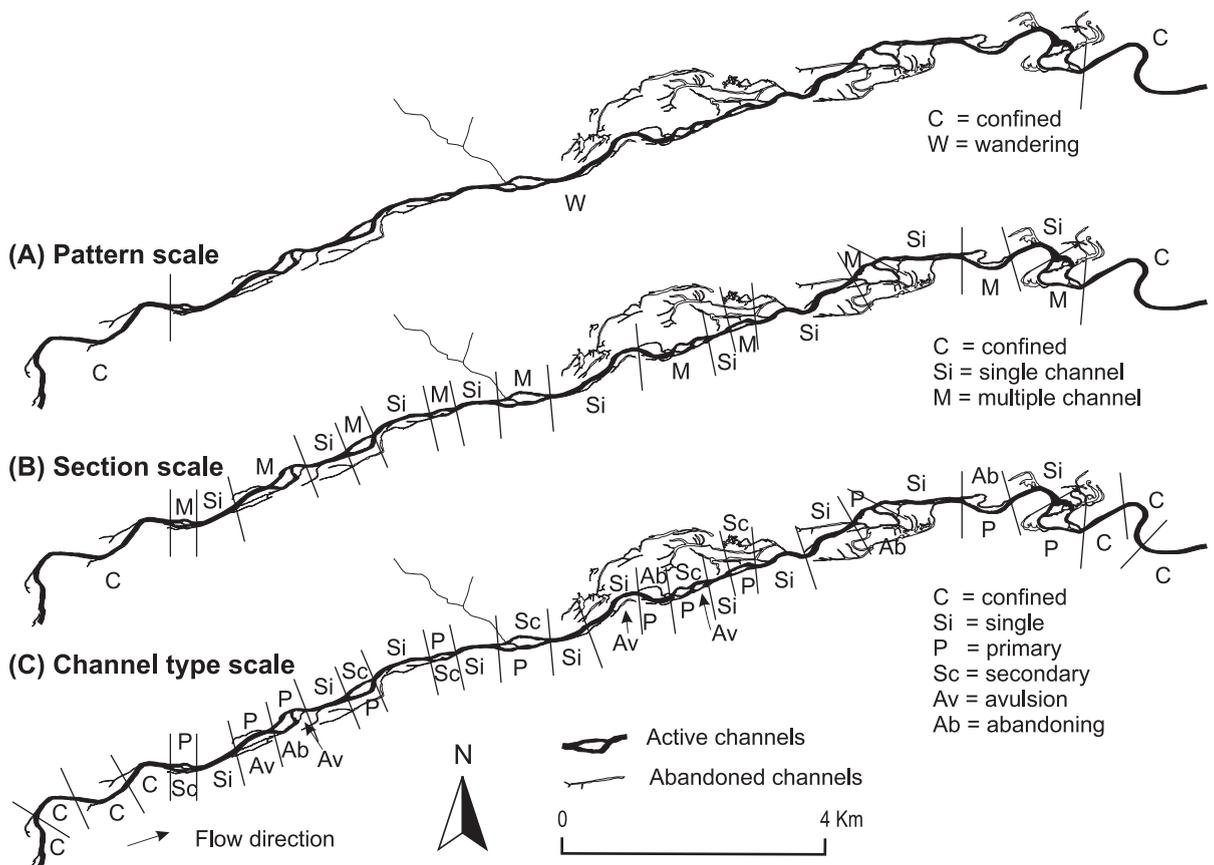
Fig. 4. Maps of classifications of channels at the (A) pattern, (B) section, and (C) channel type scales.
