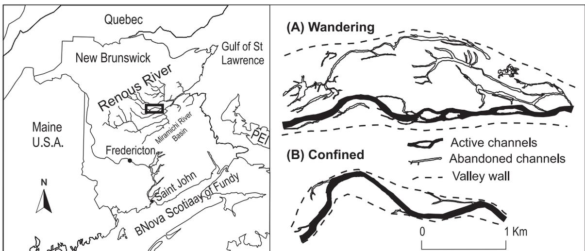
Fig. 1. Location map of the Renous River study reach. Examples of (A) wandering and (B) confined sections of the Renous River showing active channels, abandoned channels, and the location of the valley wall.
