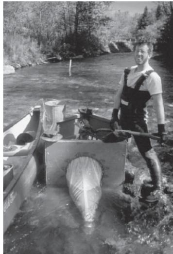
**Figure 3.** Flow isolation cell used for bulk sampling; note fines in suspension.
