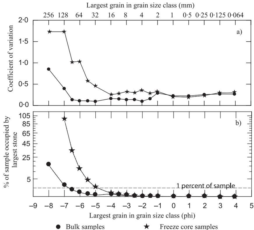
**Figure 5.** (a) Mean coefficient of variation from 12 bulk sample groups and six freeze-core sample groups (excluding data from Salmon); each group had three samples. (b) The percentage of the sample weight that the largest stone in each grain size class would contribute to the overall weight of the sample.
