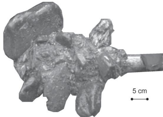
**Figure 2.** Freeze-core sample.
